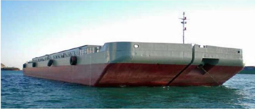
3500m3 split hopper barge non powered 78m long
